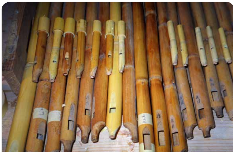
Gibilmanna. Rank of reed pipes. Note the tuning slides.
