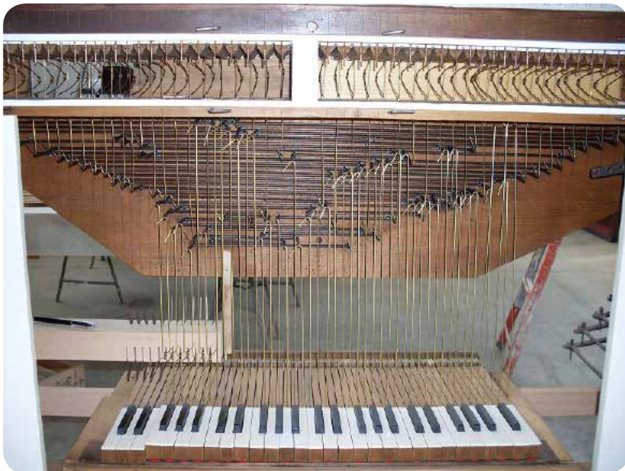
10 Detail of the tracker with the metal tracker action
